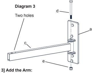
Note: Make sure the Arm Pivot Nut is tight, but still allows you to rotate the Arm.
