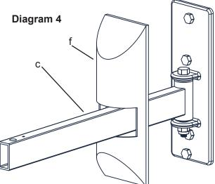
Place the round part of the Arm (c) between the tabs on the Wall Plate (a) so that two holes show on top at the other end. Place the Arm Pivot Bolt (d) down through the two tabs on the Wall Plate and through the hole in the round side of the Arm. Thread the Arm Pivot Nut (e) onto the bottom of the Arm Pivot Bolt and tighten with a wrench as shown in diagram 3.
