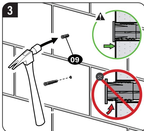
**⚠ CAUTION:** Be sure the anchors **09** are seated flush with the concrete surface.
