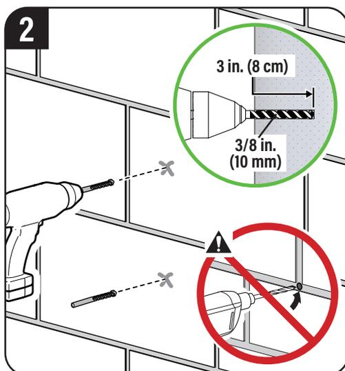
**⚠ CAUTION:** Never drill into the mortar between blocks.
