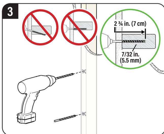
**!** **IMPORTANT:** Be sure to drill into the center of the stud.
