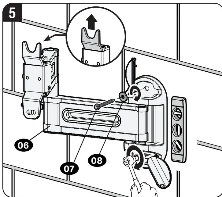
**⚠ CAUTION:** Avoid potential personal injury or property damage! Improper use could reduce the holding power of the lag screw **07**. Tighten the lag screws **07** only until they are pulled FIRMLY against the wall plate **06**. DO NOT over-tighten the lag screws **07**.
