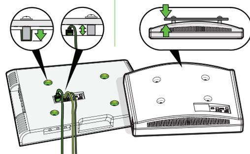
**CAUTION:** Verify adequate thread engagement with your screw **01**, washer **02**, spacer **03** combination AND TV bracket **04**.
